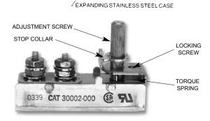
heated surface, a temperature change is sensed almost instantaneously. With an incrase in temperature, the case expands. This results in a linear change of the internal bridge assembly causing the electrical contacts to open. A decrease in temperature closes the contacts.
