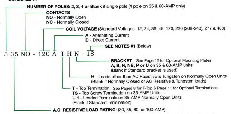
NOTES #1 Other designations are -1 thru -99. These are suffix numbers, and are reserved for units with dead special detail, construction and/or features. -11 MOV on coil (see page 29), -13 MOV & Metal Strap, -17 DIN Rail Mount, -20 DIN Rail & Metal Strap (see page 12), -18 Metal Strap (see page 7). (See example #2).
